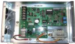
Modbus Interface TCB-IFMB641TLE
